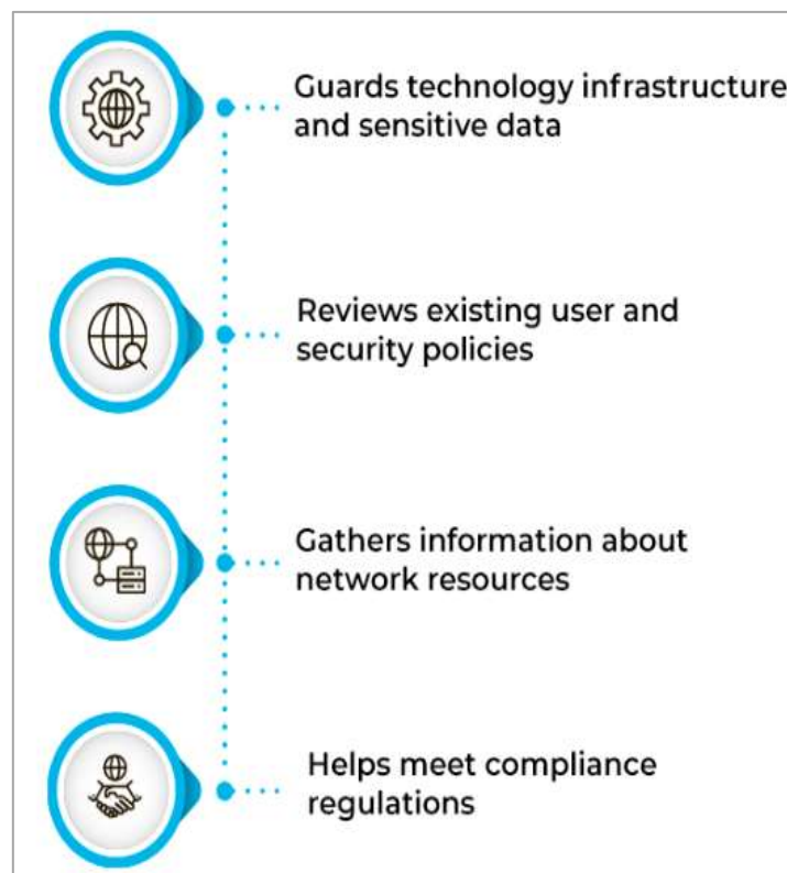
Figure 1: Basic Functions of an IDPS
