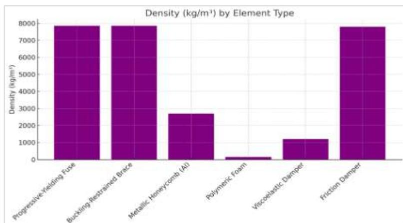
**Figure 4: Density (kg/m<sup>3</sup>) by Element Type**
