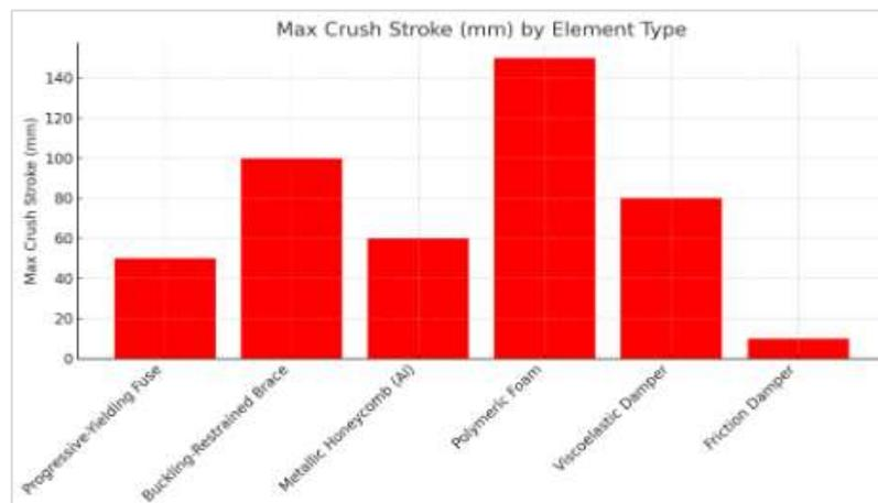
**Figure 3: Max Crush Stroke (mm) by Element Type**
