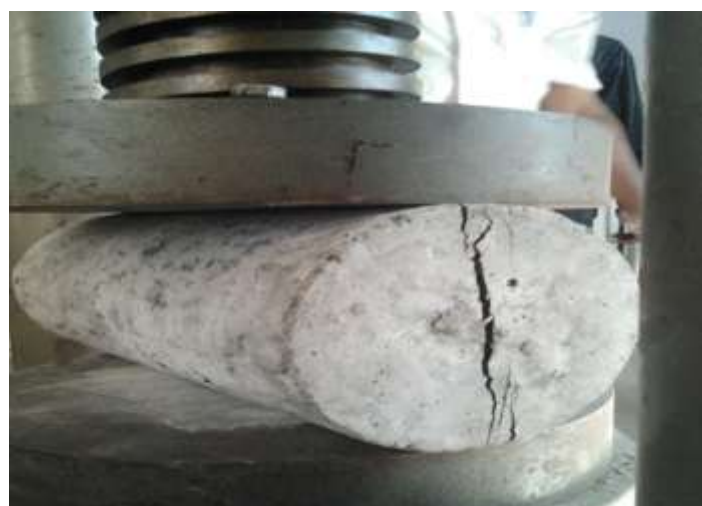
Figure: Split Tensile Test
