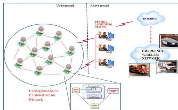
Recharging the in-ground wireless sensor networks might be a challenge. They're tough to recharge sensor batteries that have a restricted capacity. In addition, the subterranean environment makes wireless communication a problem because of the significant amount of attenuation and signal loss that occurs there.
