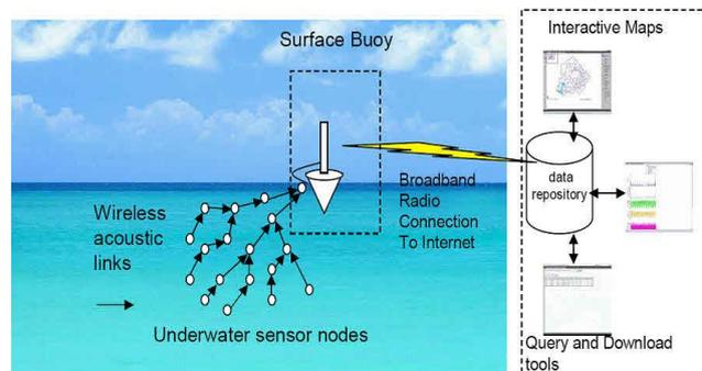
WSNs submerged in water are powered by a small, non-replaceable battery. The development of underwater communication and networking methods is necessary to address the problem of energy saving for underwater WSNs.
