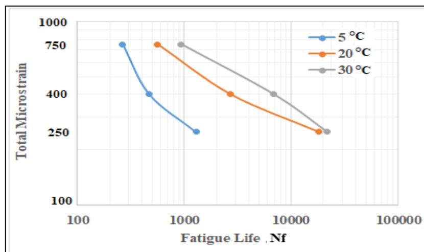
**Figure 5.** Influence of Testing Temperature on the fatigue life
