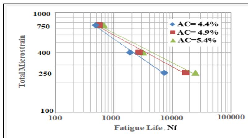
Figure 4. Influence of Asphalt Content on the fatigue life
