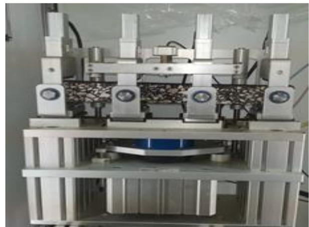
**Figure 2.** four-point bending beam test setup
