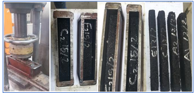
Figure 4. Preparation of the asphalt concrete beams
