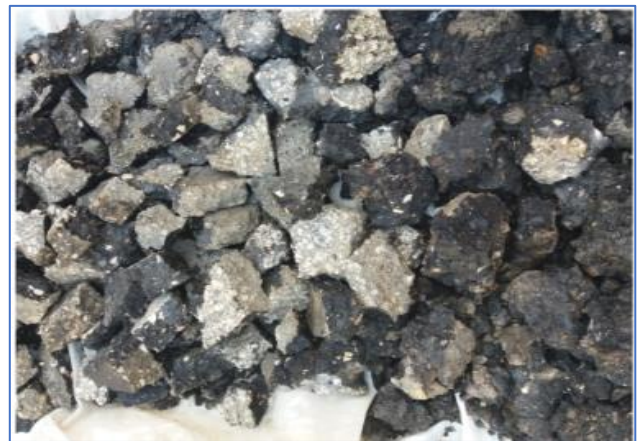
Figure 2. Reclaimed asphalt concrete (RAP).
