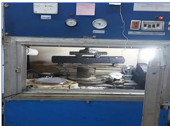
Figure 5. Beam Specimen in the PRLS testing chamber
